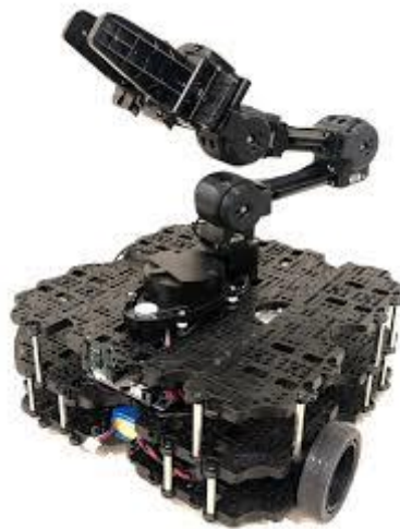
Figure 2 Turtlebot 3 with the OpenMANIPULATOR-X platform (TurtleBot3, no date)
